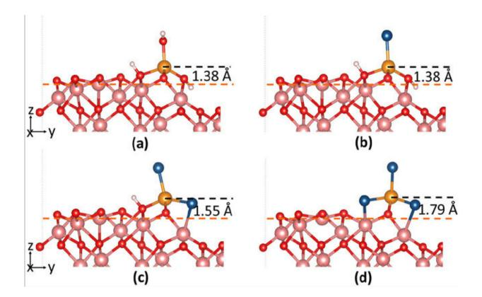
Surface structural changes to iron passive films caused by the adsorption of OH and/or Cl. (a) Fe(OH)3, (b) Fe(OH)2Cl, (c) Fe(OH)Cl2, (d) FeCl3. The location of the edge Fe atom prior to the adsorption is shown with an orange dashed line. Atoms types indicated by white (H), royal blue (Cl), large pink (Fe) and small red (O) spheres. Credit: Oregon State University College of Engineering
