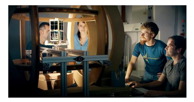
Students and staff during tests for attitude determination in space. SOMP2b uses sensors for the earth's magnetic field, the rotation rate and the sun. Credit: Götz Walter, Biermann-Jung Kommunikation & Film
