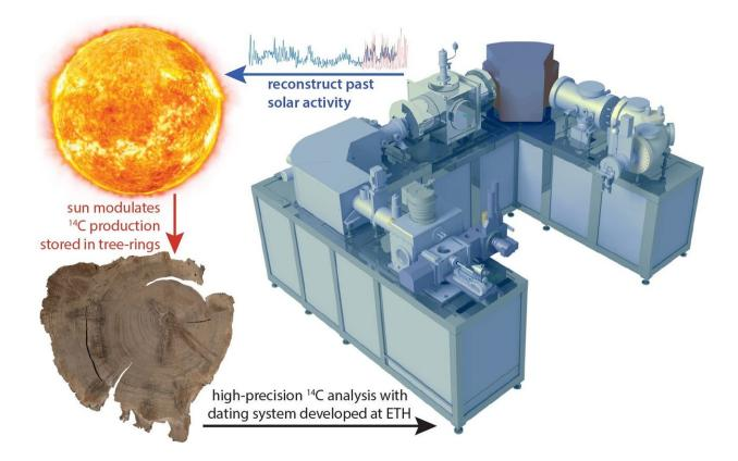
With the new instruments developed at ETH (right), researchers can measure tiny changes of a few tenths of a percent in that concentration and reconstruct pasts solar activity from them. Credit: ETH Zurich
