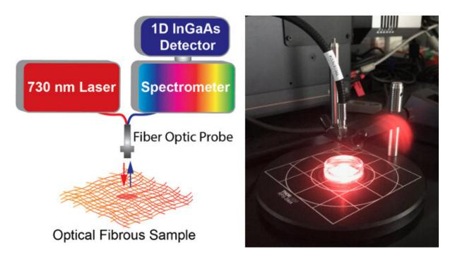
Probe system: Nanosensors are placed inside the individual fibers of a textile. Credit: Daniel Roxbury
