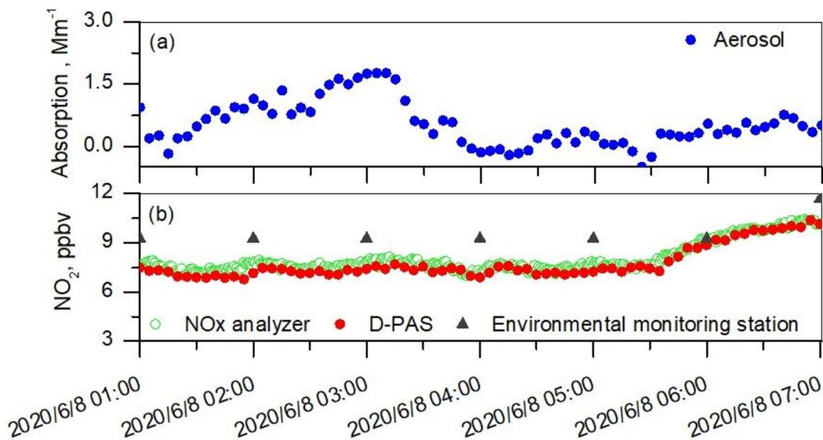
Time series measurements of aerosol absorption coefficient and NO<sub>2</sub> concentration. Credit: LIU Kun
