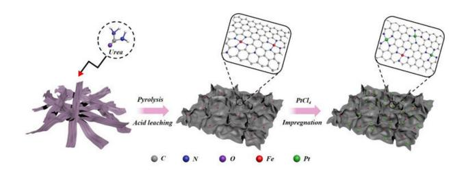
Schematic illustration for the synthesis of Fe<sub>1</sub>Pt<sub>1</sub>/NC. Credit: CAO Lijuan
