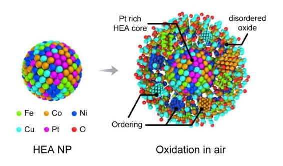
Illustration of the movement of different molecules during the oxidation of highentropy alloy nanoparticles. Credit: University of Illinois Chicago.
