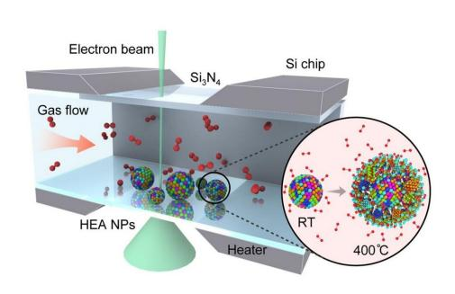
Schematic of the setup used to study the oxidation of high-entropy alloy nanoparticles (HEA NP). Inset shows HEA NP structure at room temperature (RT) and during the high-temperature oxidation. Credit: University of Illinois Chicago.
