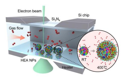
Schematic of the setup used to study the oxidation of high-entropy alloy nanoparticles (HEA NP). Inset shows HEA NP structure at room temperature (RT) and during the high-temperature oxidation. Credit: University of Illinois Chicago.
