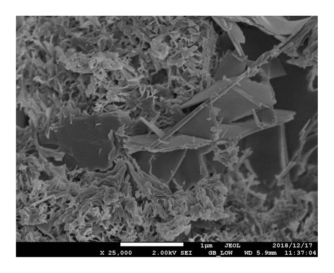
The scientists found aluminous tobermorite formed inside the walls due to reactions between minerals in the concrete mixture in the presence of water and moderately high temperatures over a prolonged period. Credit: Ippei Maruyama, Nagoya University, and Chubu Electric Power Co.
