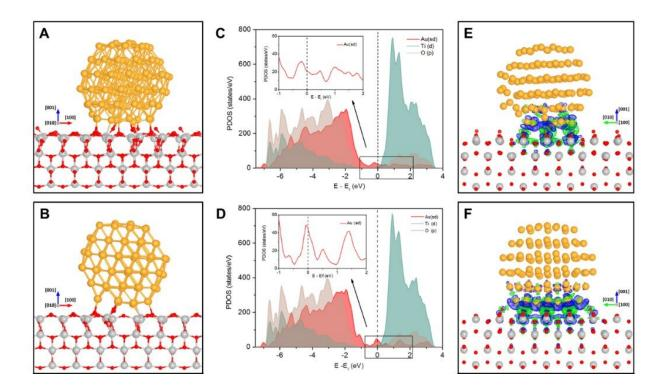
Geometric and electronic structure of Au-TiO<sub>2</sub> interface under CO/O<sub>2</sub> (A, C, E) and O<sub>2</sub> environment (B, D, F). Credit: GAO Yi
