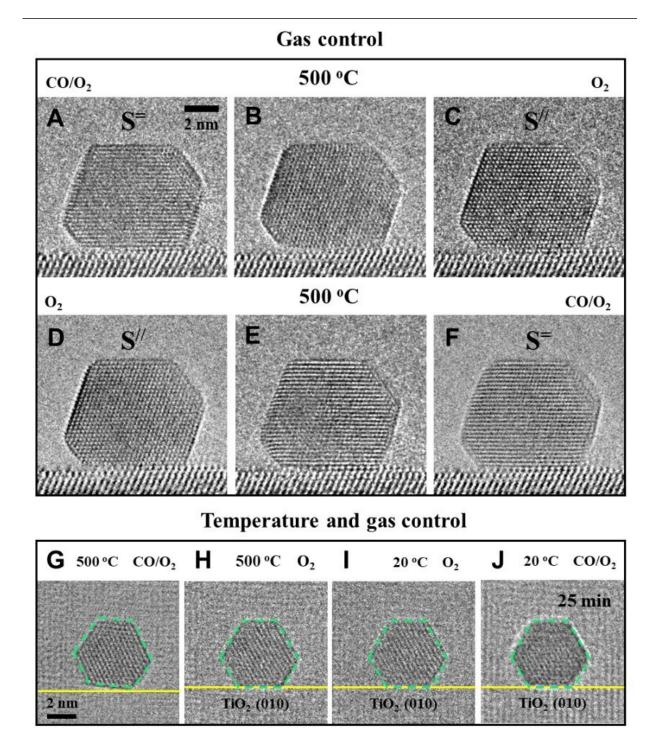
Manipulation of the Au-TiO $_2$  interface using temperature and gas control. Credit: GAO Yi
