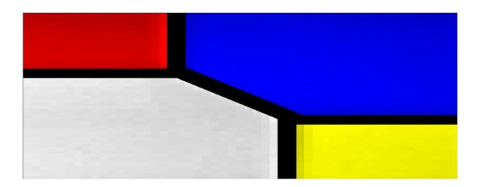
The image shows the signal measured from a charge sensor, where the scientists have mapped the signal values to colours. Different colours correspond to different configurations of electrons on the quantum dot array. The black lines correspond to transitions of electrons, where the black diagonal line corresponds to a cascade of transitions. Credit: C.J. van Diepen
