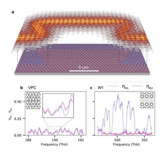
a, 3D rendition of the scanning electron micrograph of the VPC with a trapezoidal ( $\Omega$ -shaped) structure along the domain wall, comprising four sharp corners and the two parity-inverted VPCs shown in false colors. The upper extension shows the full two-dimensional real-space amplitude map of the propagating edge state. b, Calculated backward/forward energy ratio before
