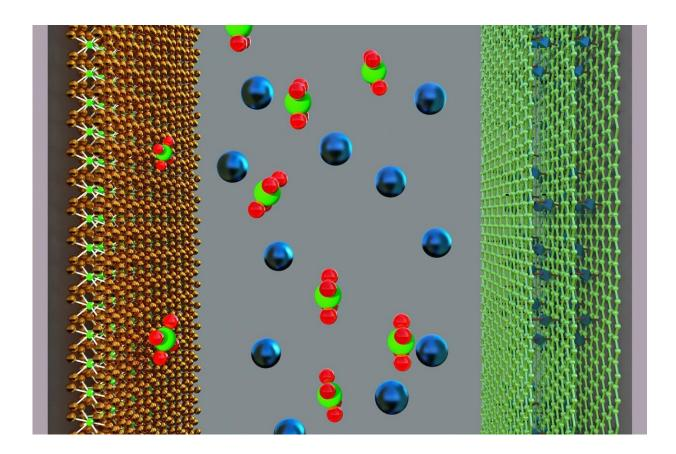
Graphene hybrids made from metal organic frameworks (MOF) and graphenic acid make an excellent positive electrode for supercapacitors, which thus achieve an energy density similar to that of nickel-metal hydride batteries. Credit: Prof. Dr. Jayaramulu Kolleboyina/IITJ
