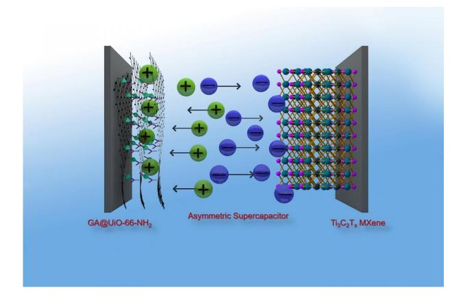
Graphene hybrid made from metal organic frameworks (MOF) and graphenic acid make an excellent positive electrode for supercapacitors, which thus achieve an energy density similar to that of nickel-metal hydride batteries. Credit: Prof. Dr. J. Kolleboyina/IITJ
