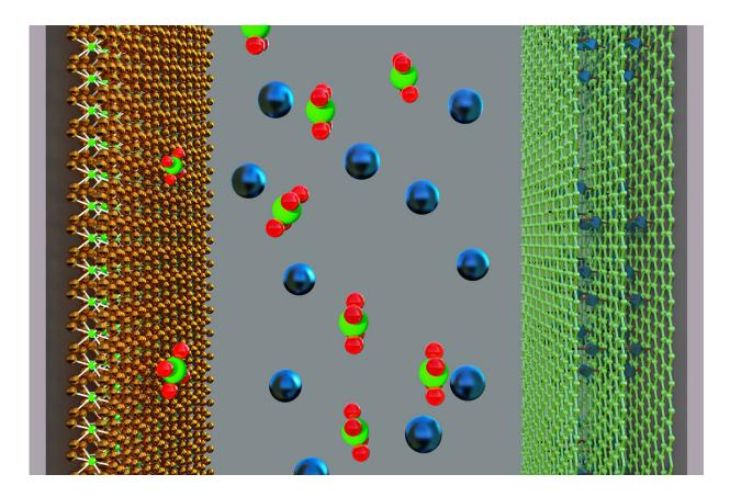
Graphene hybrids made from metal organic frameworks (MOF) and graphenic acid make an excellent positive electrode for supercapacitors, which thus achieve an energy density similar to that of nickel-metal hydride batteries. The black color indicates high electron mobility within the material. Credit: Prof. Dr. J. Kolleboyina / IITJ
