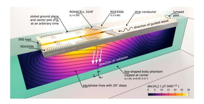
The exciting slotted microstrip line radiates into a box-shaped human body phantom for body MRI RF excitation. The color plot shows the normalized magnitude of the simulated Hx distribution, while black contours represent wavefronts in the conductive medium. Calculated surface current density distribution on the slotted ground plane is shown with black arrows.Nature Communications (2021). DOI: 10.1038/s41467-020-20708-w
