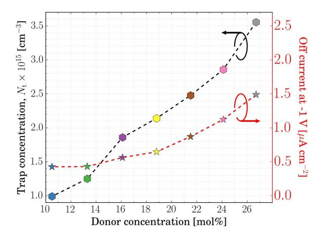
By modelling the dark current of several donor-acceptor systems, Mr. Kublitski reveals the interplay between traps and charge-transfer states as the source of dark current and shows that traps dominate the generation processes in the dark. Credit: Jonas Kublitski
