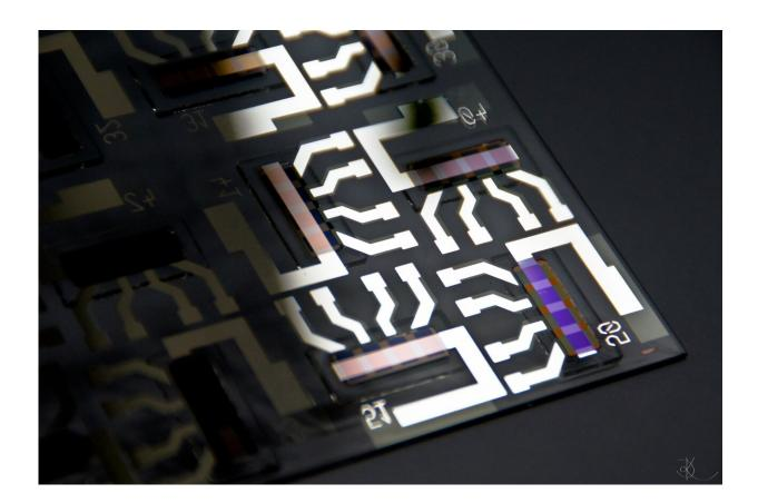
Flexible organic photodetectors (OPDs) have a huge potential for applications in low-cost imaging, health monitoring and near infrared sensing. Credit: Christian Körner
