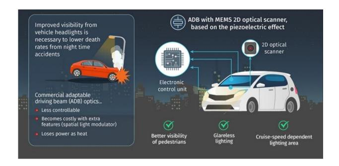
Headlights Infographic: ADB with MEMS 2D optical scanner, based on the piezoelectric effect. Credit: SPIE
