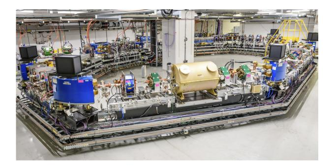
Fermilab's optical stochastic cooling experiment is now under way at the 40-meter-circumference Integrable Optics Test Accelerator, a versatile particle storage ring designed to pursue innovations in accelerator science. Credit: Giulio Stancari, Fermilab
