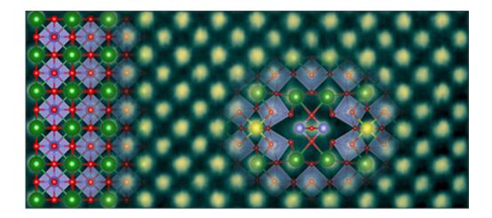
Using advanced analytical scanning transmission electron microscopy (STEM) at a magnification of 10 million times, University of Minnesota researchers were able to isolate and image the structure and composition of the metallic line defect in a perovskite crystal BaSnO3. This image shows the atomic arrangement of both the BaSnO3 crystal (on the left) and the metallic line defect. Credit: Mkhoyan Group, University of Minnesota
