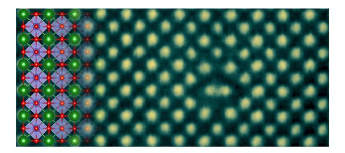
University of Minnesota Professor K. Andre Mkhoyan and his team used analytical scanning transmission electron microscopy (STEM), which combines imaging with spectroscopy, to observe metallic properties in the perovskite crystal barium stannate (BaSnO3). The atomic-resolution STEM image, with a BaSnO3 crystal structure (on the left), shows an irregular arrangement of atoms identified as the metallic line defect core. Credit: Mkhoyan Group, University of Minnesota
