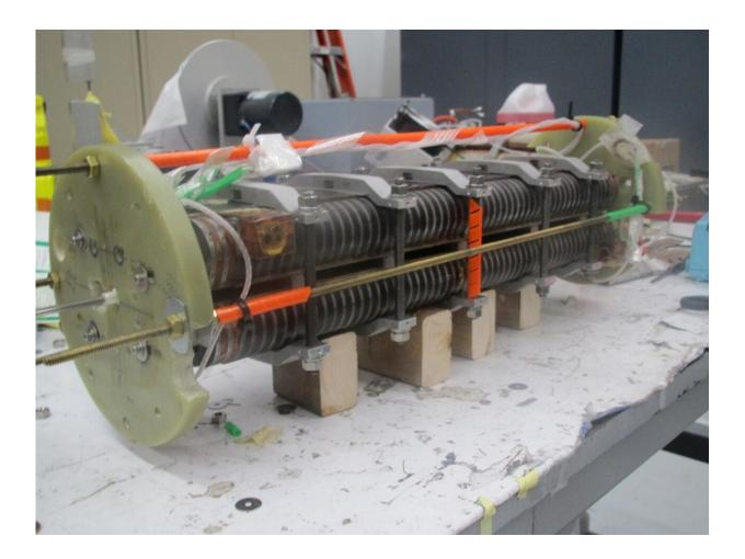
This half-meter-long prototype of a niobium-tin superconducting undulator magnet was designed and built by a team from three U.S. Department of Energy national laboratories. The next step will be to build a meter-long version and install it at the Advanced Photon Source at Argonne. Credit: Ibrahim Kesgin, Argonne National Laboratory
