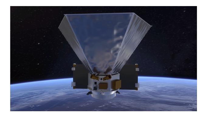
This animation shows the preliminary design for the spacecraft, including hexagonal sun shields that will help keep the instruments cool. Credit: NASA/JPL-Caltech
