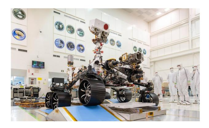
In a clean room at NASA's Jet Propulsion Laboratory in Southern California, engineers observed the first driving test for NASA's Mars 2020 Perseverance rover on Dec. 17, 2019. Credit: NASA/JPL-Caltech
