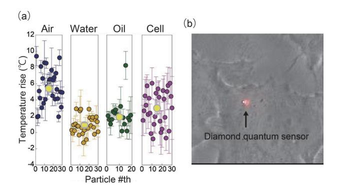
(a) Temperature increases observed with hybrid sensors in air, water, oil, and inside cell. These results are consistent with the idea that higher temperature increases occur in solvents with smaller thermal conductivities. The literature values for the thermal conductivities of air, water, and oil are 0.026, 0.61, and 0.135 W/m\* K, respectively. (b) Bright field microscopic image of a HeLa cell with a hybrid sensor inside. Credit: Osaka University
