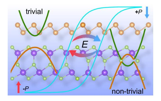
Rice University materials theorists show how a unique two-dimensional compound of antimony and indium selenide can have distinct properties on each side, depending on polarization by an external electric field. The figure indicates that two states for nonvolatile memory devices can be flipped by the polarization of the ferroelectric layer. Credit: Illustration by Jun-Jie Zhang
