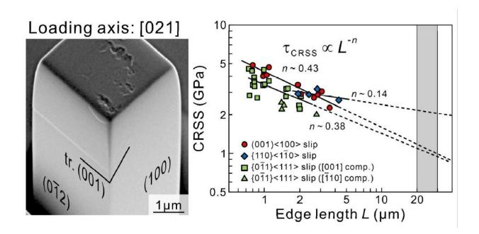
The scientists measured the plastic deformation that happened when a tiny probe exerted force on the micropillar specimens with various loading axis orientations. Credit: National Institute for Materials Science (NIMS)
