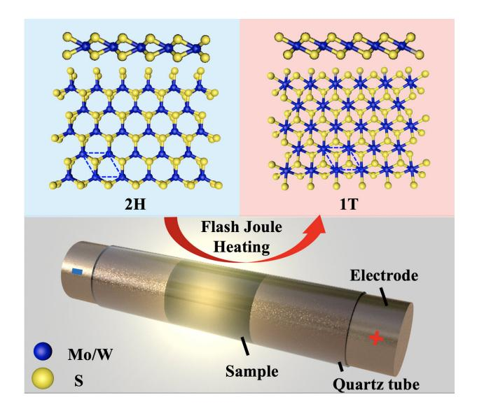
Rice University scientists extended their technique to produce graphene in a flash to tailor the properties of 2D dichalcogenides molybdenum disulfide and tungsten disulfide, quickly turning them into metastable metallics for electronic
