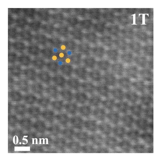
An electron microscope image shows tungsten disulfide in its metastable 1T state. The orange dots represent sulfur atoms, the blue represent tungsten. Rice University scientists used flash Joule heating to tailor the properties of 2D dichalcogenides, quickly turning them into metastable metallics for electronic
