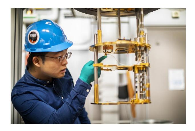
Thermal testing of the new metamaterial tiles in an advanced cryogenic facility showed that they could be effectively cooled to the cryogenic temperatures necessary. Credit: Eric Sucar, Penn Today
