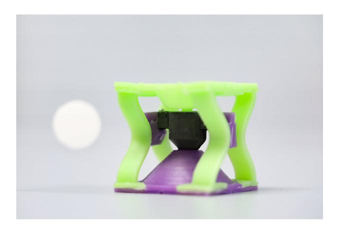
The metamaterial developed by EPFL scientists is made of silicon and magnetic powder and has a complicated structure that allows mechanical properties to vary. Credit: © Alain Herzog / 2021 EPFL
