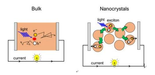
In bulk, excitation by light creates charges (electron and hole), which diffuse to their respective electrodes to be extracted as electric current. In nanocrystals, excitation by light creates excitons, which travel via energy transfer. The excitons dissociate at the electrodes and extracted as electric current. Credit: Tze Chien Sum
