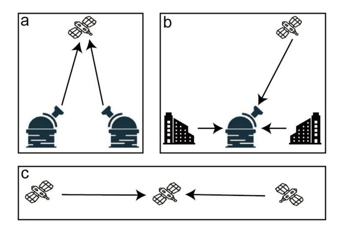
Possible configurations of satellite-based MDI-QKD. (a) the satellite plays the role of the detection terminal, while two ground stations send photons via the uplink to the satellite. (b) A ground station plays the role of the detection terminal. Users in the ground fiber-based network share secret keys with the satellite via the ground station. (c) MDI-QKD between three satellites. Credit: Cao et al.
