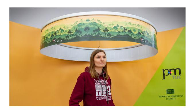
Printed speakers create surprising jungle illusion. Printed electronics embedded in a paper web enable 360° surround sound. Varvara Bachul from the Institute of Print and Media Technology at Chemnitz University of Technology analyzes the sound generated inside the T-RING. The sounds come from 56 printed individual loudspeakers that are connected to form seven segments on the circular track, which is almost four meters long. Photo: Jacob Müller
