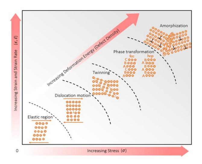
Proposed hierarchical deformation mechanism paradigm for the equi- atomic CrCoNi-based HEAs subjected to increasing degrees of deformation. Elastic deformation, dislocation-mediated plasticity, twinning-induced plasticity, TRIP, and finally solid-state amorphization. Triggering the next mechanism re- quires
