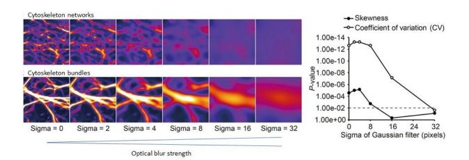
Optical blur was artificially added to microscopic images of reticular and bundle cytoskeleton and the difference between the existing and proposed methods was assessed. In the right figure, the higher the vertical axis, the better the distinction between the two. The proposed method more accurately distinguishes the reticular and bundle cytoskeleton images, even in degraded images, compared to the existing method. Credit: Associate Professor Takumi Higaki
