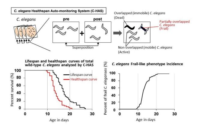
C-HAS can distinguish between nematodes that are alive, dead, or in an inactive state of survival by using superimposed periodic (before & after) images. Credit: Associate Professor Tsuyoshi Shuto
