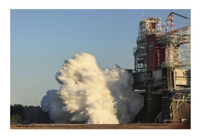
In this Saturday, Jan. 16, 2021 photo made available by NASA, the core stage for the first flight of NASA's Space Launch System rocket undergoes a hot fire test at NASA's Stennis Space Center near Bay St. Louis, Miss. All four corestage engines fired for barely a minute, rather than the intended eight minutes. On Tuesday, Jan. 19, 2021, NASA blamed the automatic shutdown on the strict test limits. (Robert Markowitz/NASA via AP)
