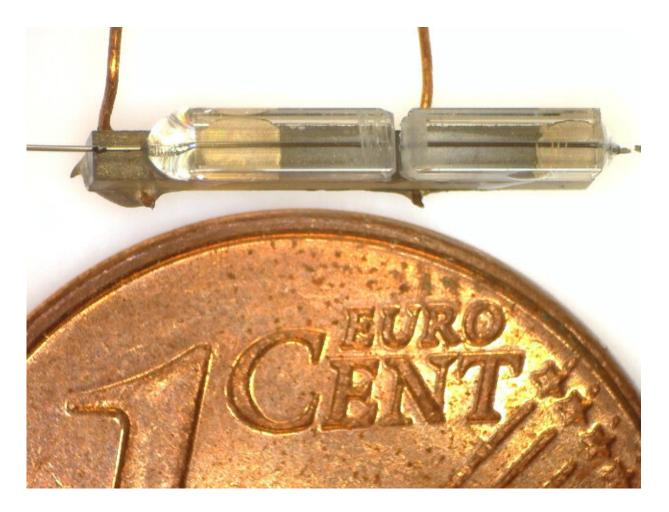
The miniaturized optical filter is located in the central slot of the sleeve mount. Credit: © Uni Bonn
