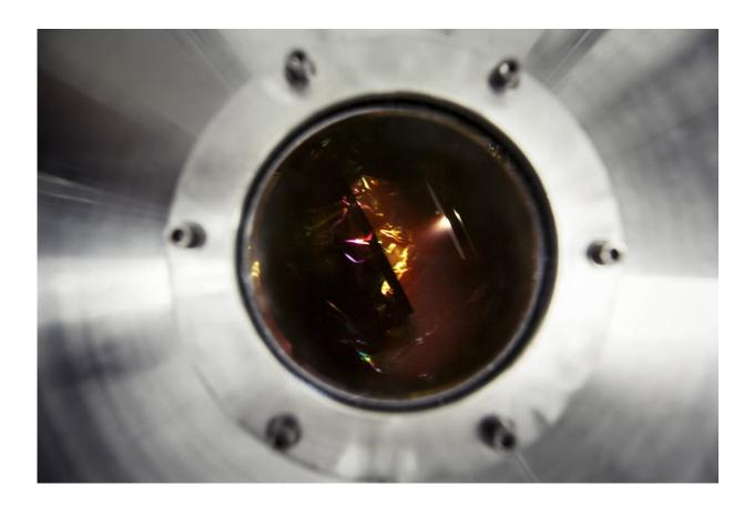
View through a window of the interior of an ultra-high vacuum reactor where TiO2 nanotubes are decorated with CoO nanoparticles. We see the flame (plasma produced by laser ablation) that sputters the CoO to give rise to the formation of its nanoparticles. Credit: Christian Fleury (INRS)
