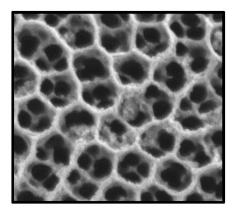
Electron microscopy image (top view) of an array of TiO2 nanotubes (like honeycomb cells of a bee hive) decorated with cobalt oxide (CoO) nanoparticles (NP). Credit: INRS
