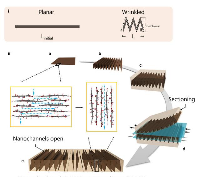
Vertically aligned Zr-GO/epoxy membrane (VAGME)
