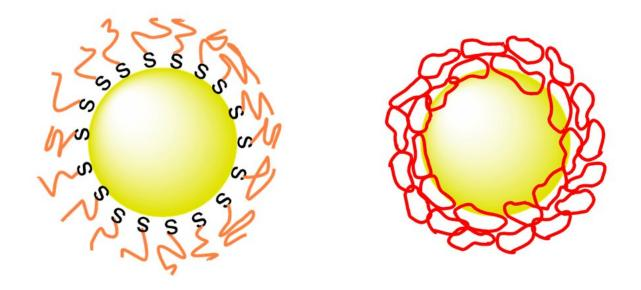
A comparison of how linear PEG (left) and cyclic PEG (right) attach to a gold nanoparticle. Credit: Yubo Wang, Takuya Yamamoto
