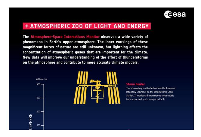
The Atmosphere-Space Interactions Monitor (ASIM) is a collection of optical cameras, photometers and an X- and gamma-ray detector designed to look for electrical discharges born in stormy weather conditions that extend above thunderstorms into the upper atmosphere. Credit: ESA
