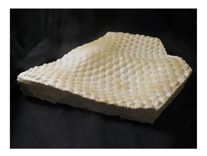
Mycolite panels are made by pouring the composite into a mould. Credit: FUNGAR/CITA, 2019-2020
