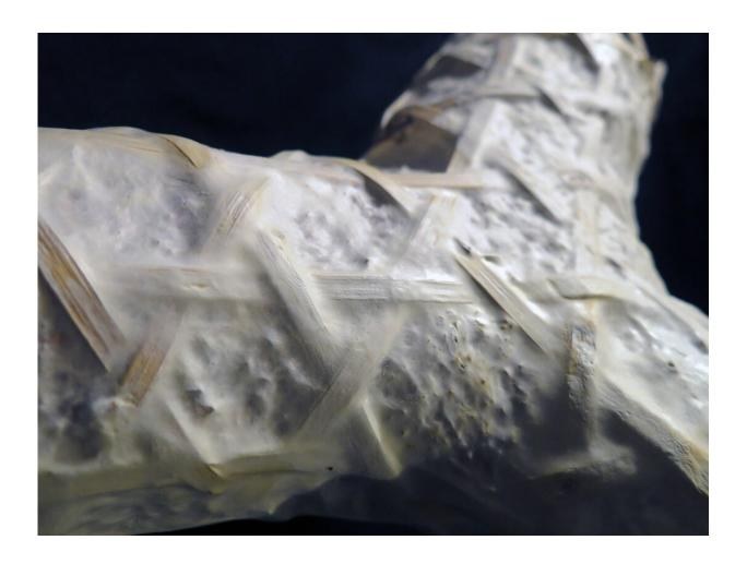
The mycelium composite can be grown over a woven scaffold for a period of 7-10 days, eventually encasing the structure. Credit: FUNGAR/CITA, 2019-2020
