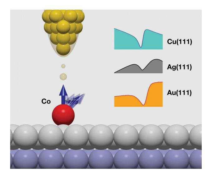
Illustration showing the atomic tip of a scanning tunneling microscope while probing a metal surface with a cobalt atom positioned on top. A characteristic dip in the measurement results is found on surfaces made of copper as well as of silver and gold. Credit: Forschungszentrum Jülich
