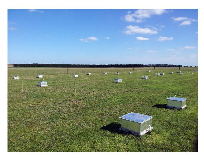
Static chambers are used in fields to measure greenhouse gases. This helps scientists determine the effect of fertilizers on improving nitrogen use efficiency. Credit: Shu Kee Lam
