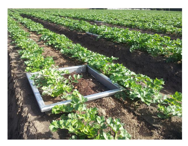
To measure greenhouse gas emissions from manure application on a celery farm, researchers covered some of the plants with chambers that would trap the gases. The metal border is the base of the chamber. Credit: Shu Kee Lam
