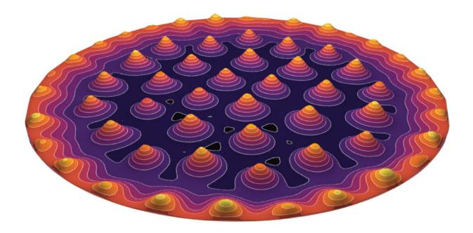
When a magnet is brought close to a ferrofluid, the ferrofluid shape-shifts to form spikes that align with the magnetic field. Credit: Huang et al.
