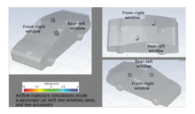
Computational fluid dynamics simulation of airflow in cars with two windows, one rear, one front, open. Credit: Varghese Mathai CC-BY-ND
