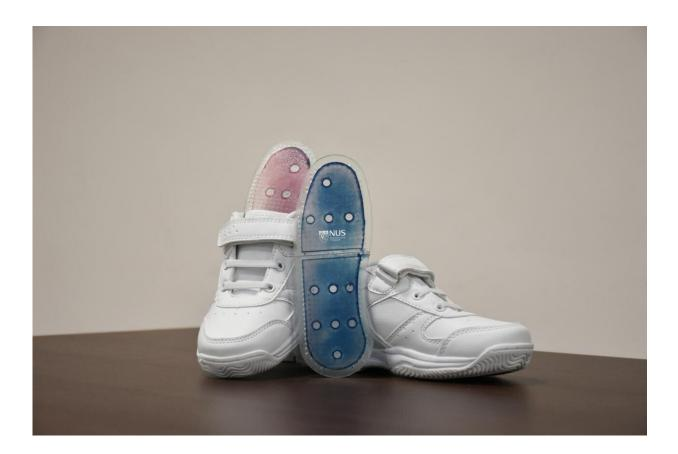
A team of researchers from the National University of Singapore invented a novel thin film that evaporates sweat six times faster and holds 15 times more moisture than conventional materials. In this prototype, the insole coated with the novel thin film turns from blue to pink as it absorbs moisture. The insole can be easily 'regenerated' by putting it under the sun, and be reused for more than 100 times. Credit: National University of Singapore
