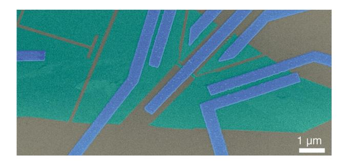
False-colour electron microscope image of the sample, the green layers are graphene on top of the grey superconductor. The blue metal electrodes are used to extract the entangled electrons. Credit: Aalto University
