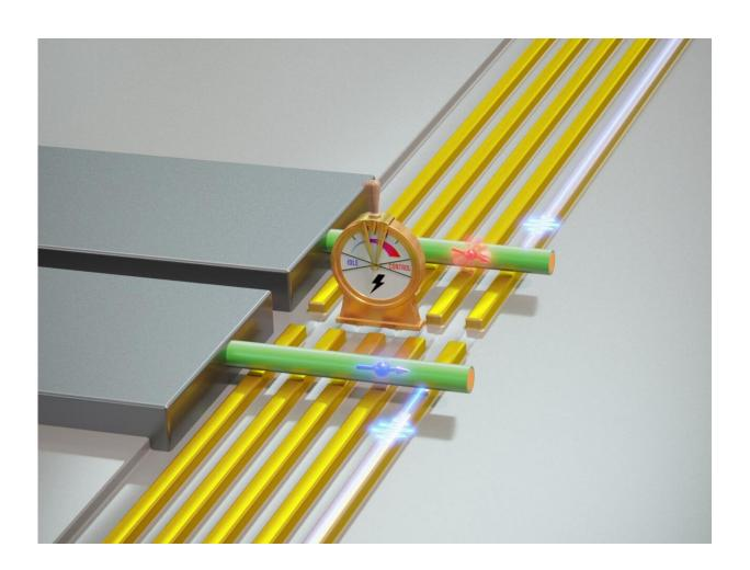
A nanowire made of germanium and silicon (blue/green) lies on electrodes known as gates (gold). Voltages applied to the gates lead to the formation of individual spin qubits (blue and red arrows) that can be manipulated by microwave signals (blue pulse). In one mode, the qubit is slow and the quantum information is more stable (blue spin). In the other, the qubit can be changed more quickly (red spin). Credit: University of Basel, Department of Physics
