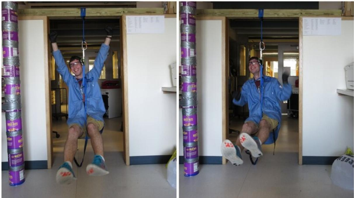
Nicholas Belloch, Guarini '21, shows off a temporary glue that is strong enough to hold a PhD candidate, but can be released without force. For this photo, the glue was applied between the carabiners on two separate pieces of aluminum metal, one piece tied to the wooden support, the other attached to a rock-climbing harness. Credit: Nicholas Belloch, Guarini '21
