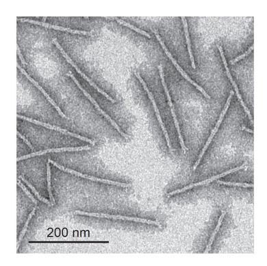
Using DNA origami as a platform to build superconducting nanoarchitectures. Transmission electron microscopy (TEM) image of DNA origami wires before the coating. Credit: Lior Shani, Philip Tinnefeld, Yafit Fleger, Amos Sharoni, Boris Shapiro, Avner Shaulov, Oleg Gang, and Yosef Yeshurun
