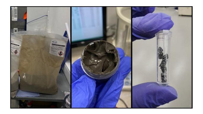
Figure 1. From left to right: lunar regolith simulants, resulting paste, and stereolithographic printed samples. Credit: Skolkovo Institute of Science and Technology
