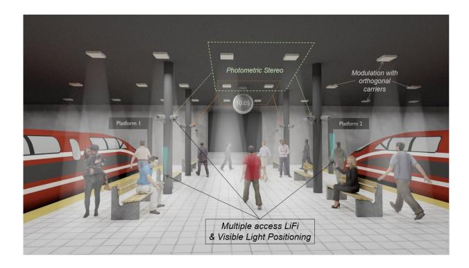
In a public area, LEDs could be used for general lighting, visible light communication and 3D video surveillance. The illustration shows multiple access LiFi -- wireless communication technology that uses light to transmit data and position between devices -- and visible light positioning in a train station. Credit: Emma Le Francois, University of Strathclyde
